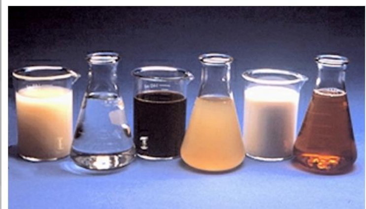
Fig. 6-1. Liquid admixtures, from left to right: antiwashout admixture, shrinkage reducer, water reducer, foaming agent, corrosion inhibitor, and air-entraining admixture. (69795)
