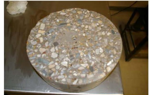
Sample After 6 Cycles (Each Cycle is 12 Hours)
