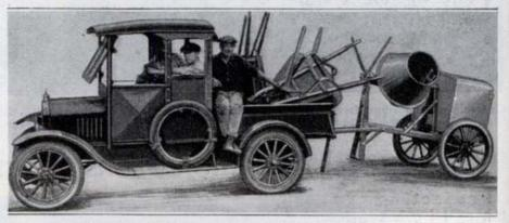
Concrete Mixer Mounted on a Rubber-Tired Two-Wheeled Truck, Which can be Hauled behind an Auto Truck at a 30-Mile Pace Instead of the Usual 10 Miles an Hour
