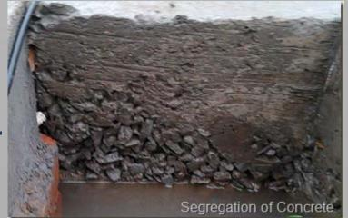
the denser aggregates settle to the bottom while the lighter cement paste tends to move upwards
