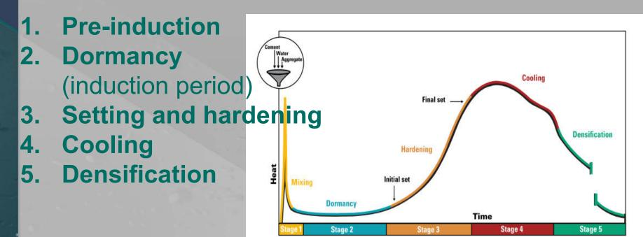
Figure 4-2. General hydration curve delineating the five stages
