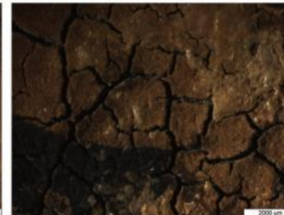
(f) Drying after 90 days corrosion
