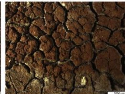
(h) Drying after 180 days corrosion
