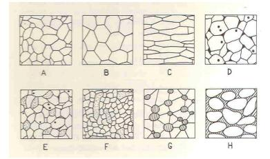
Fig. 1: Idealized microstructures: A) poly-crystallic with grains of different dimension,
