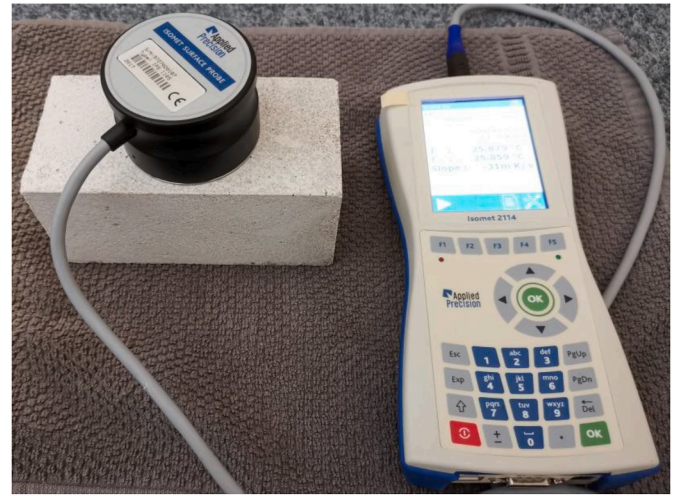
Fig. 8. Experimental determination of thermal conductivity of the reference sample at room temperature using a transient heat pulse method.
