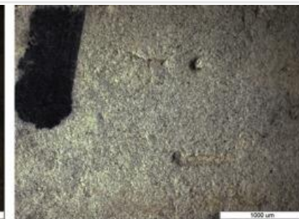
(b) Drying after 7 days corrosion
