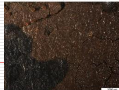
(g) After 180 days corrosion
